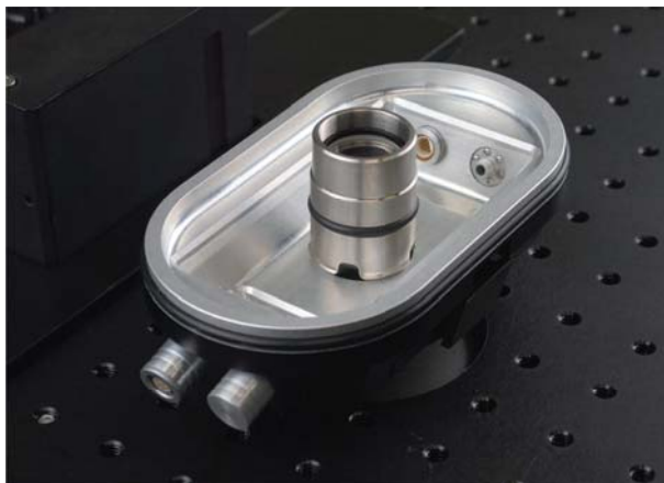
Figure 2: View showing the wired access port (cover removed) and interchangeable adapters for electrical or optical applications.
