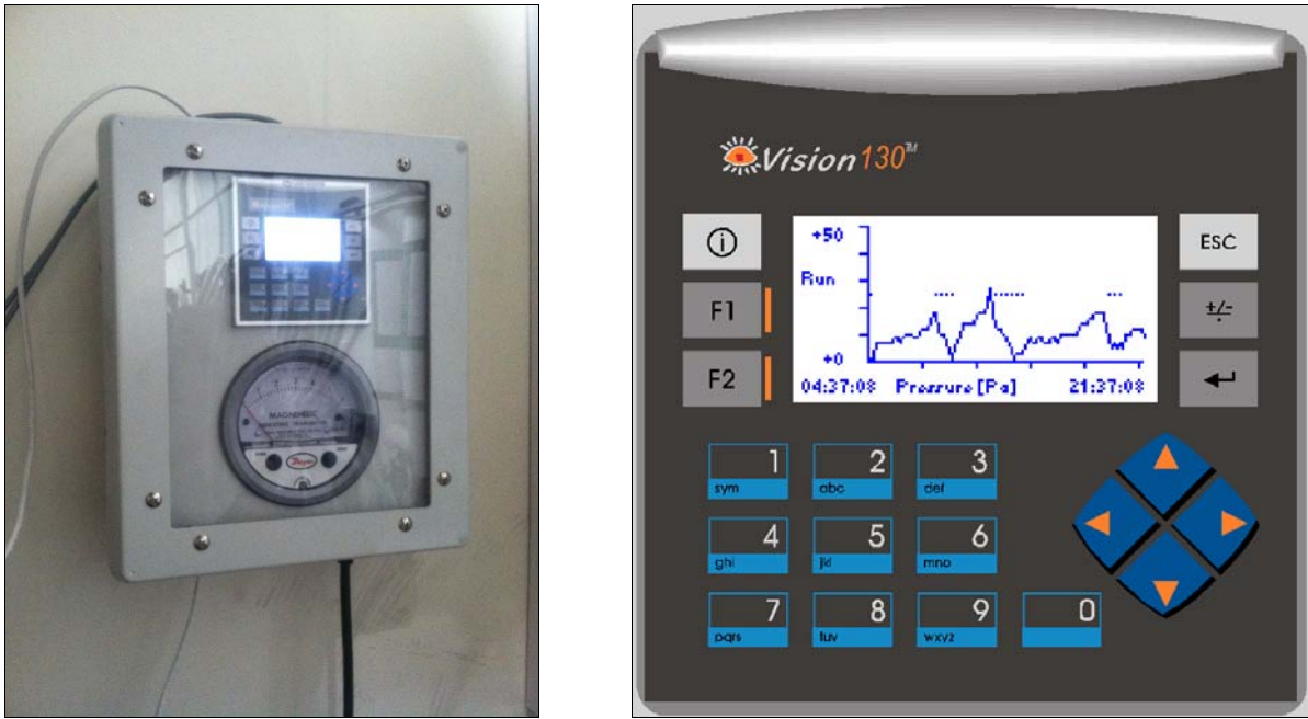
Figure 4 (left) Gas bag and compressor controller (right) GUI of the controller showing log graph
