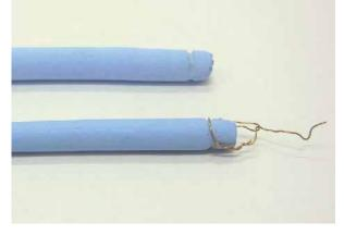
Groove cut at end of feed rod for later wiring.
