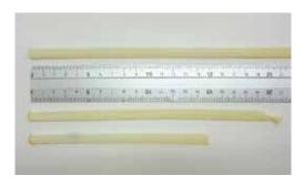
1. Cut suitable length of rubber tube and tie off one end.
