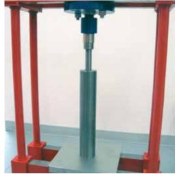
4. Insert piston into the pressure vessel. Set into press unit and apply desired load.
