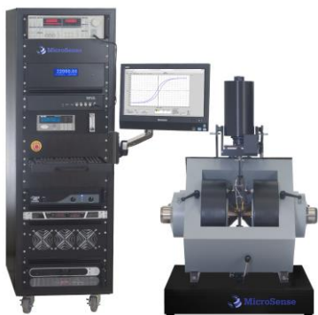
Even the high field EZ11 has a small footprint thanks to the single cabinet design enabled by the compact magnet power supply.
