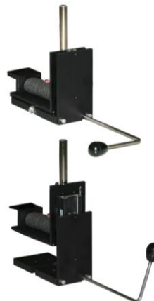
Temperature chamber in down position for room temperature measurements
