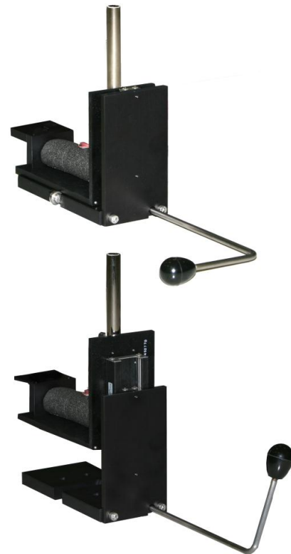
Figure 1. The temperature chamber is mounted on a slide that allows the user to bring the chamber in place in seconds when needed and move it out of the way easily to quickly change samples.
