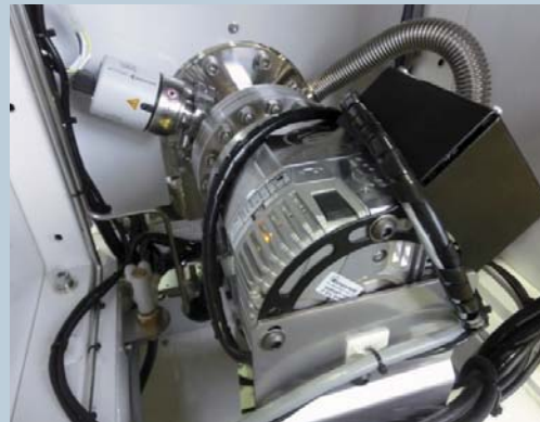
TMP directly connected to 4" gate valve
